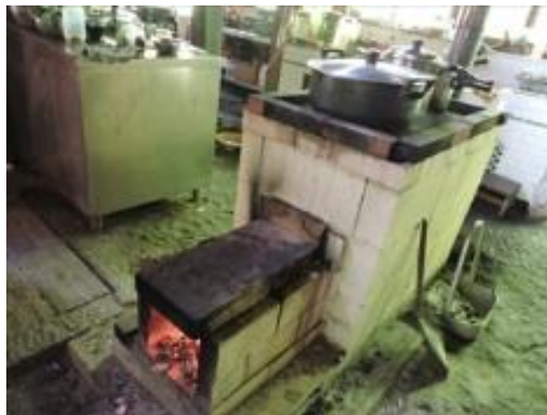
My rocket kitchen stove, developed by a friend who runs a natural farm nearby
